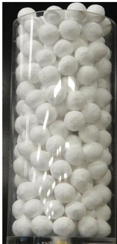
Figure B-7: Polymer encapsulated PCM
