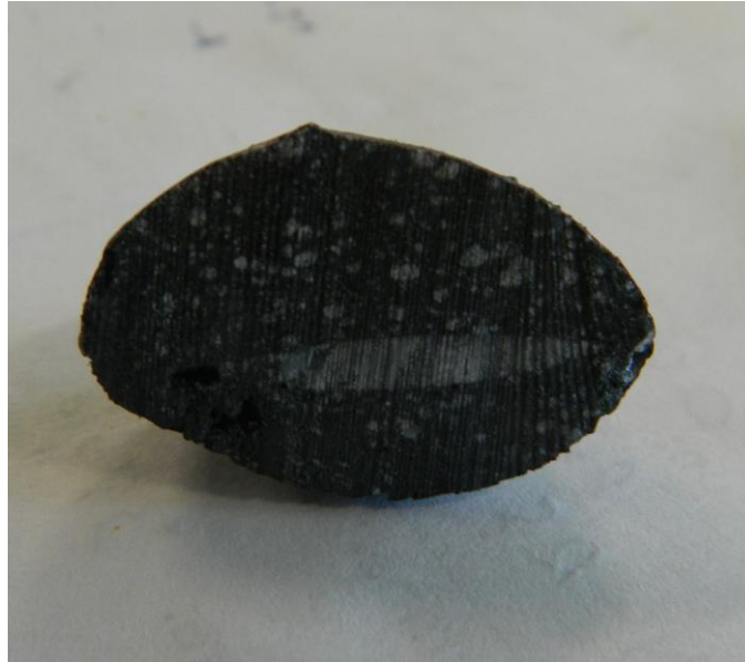
Figure 5-9: 5 wt% of graphene dispersed in NaNO 3 capsule
