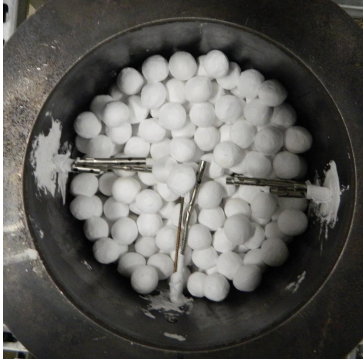
Figure B-8: Randomly packed capsules inside the packed-bed
