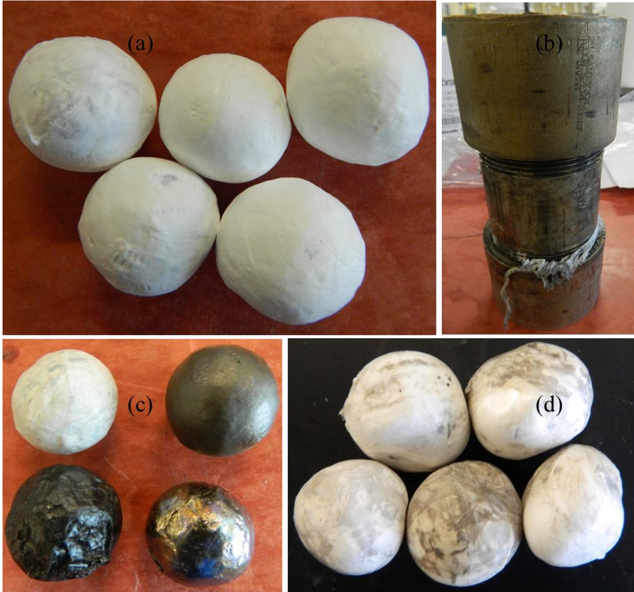
Figure 3-19: a) Polymer-coated capsules at zero cycle b) Steel cylinder filled with oil for thermal cycling c) Metal and polymer coated capsules after 1000 cycle d) Polymer coated capsules after 1000 thermal cycle
